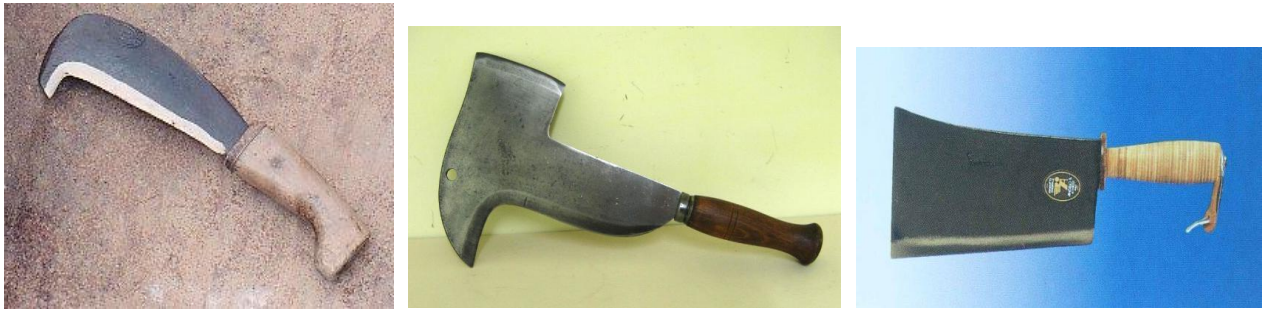
Above: (left) a roncola from Rome known locally as MARRACCIO (a design unchanged since the Roman period, see below); (centre) a pennato from Terni in Umbria; (right) a manaresso by Angelo-B
